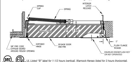
NOTE: For fire-rated ceiling access doors, on size 16" x 16" and larger, extra spring supplied with door must be attached from back of door pan to framing or floor above. In horizontal (ceiling) applications door has self-assisted closing.
