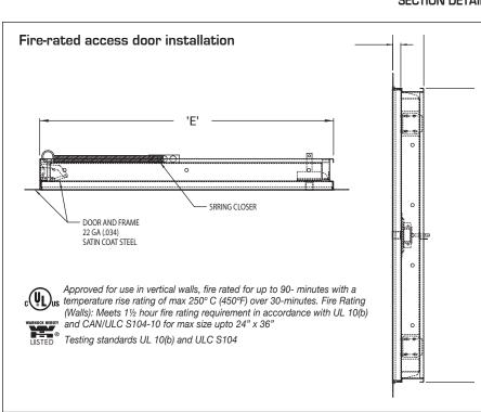
FIRE RATED Recessed for drywall walls For installation in drywall walls requiring concealing of the door panel consistent to surroundings.
