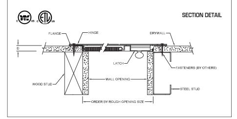
The FR SMP 840 is designed to maintain the continuity of a fire barrier when installed in a vertical separation. The assembly is manufactured under the factory inspection service of Intertek (Warnock Hersey) and has a label reading: "Listed access frame and fire door assembly. 2 hour fire rating. Vertical installation only. No temperature rise rating"
