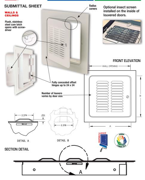
This Premium precision-flush access door for wall and ceiling installation promotes air flow and temperature control with louvered options
