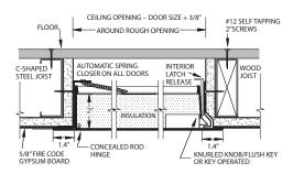
**NOTE:** For fire-rated ceiling access doors, on size 16" x 16" and larger, extra spring supplied with door must be attached from back of door pan to framing or floor above. In horizontal (ceiling) applications door has self-assisted closing.
