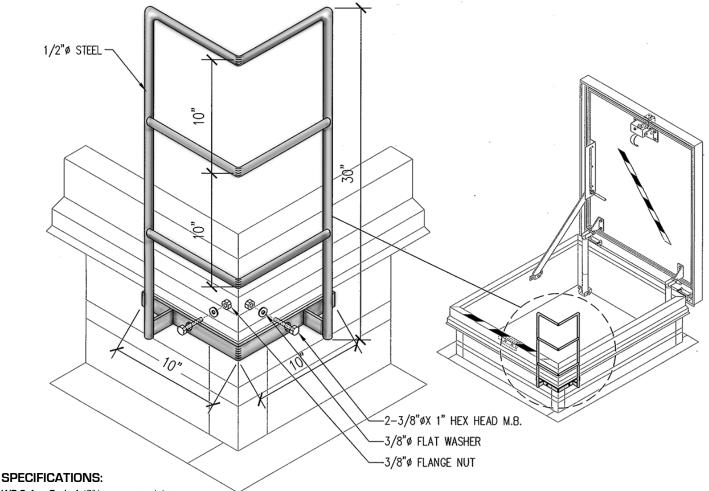
WB Safety Grab: 1/2" heavy ga. steel that attaches to the roof hatch
