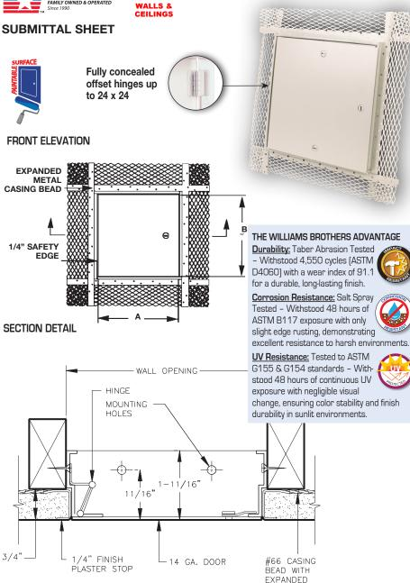
Designed for all plaster walls and ceilings. The 1/4" safety edge gives the door a strong frame and prevents the plaster from being chipped under normal use.
