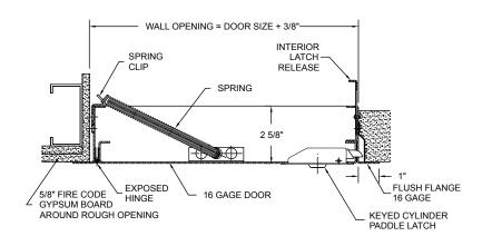
**NOTE:** For fire-rated wall access doors, on size 16" x 16" and larger, extra spring supplied with door must be attached from back of door pan to framing or floor above. In horizontal (ceiling) applications door has self-assisted closing.
