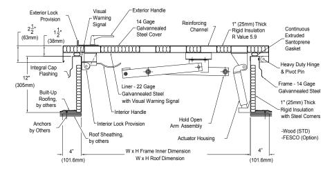
This newly re-designed WB Roof Hatch offers improved features such as a heavy duty lock and handle assembly, heavy gauge, weather-resistant gasket and fully concealed hinge hardware located on the interior making rust unlikely. Pre-lubricated compression springs, encased in zinc-plated telescopic tubes held in place by 3-sided welded brackets. Durable and re-coatable gray primer finish comes standard.
