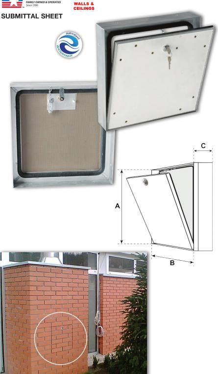
The WB EXT-DWAL 1650 is a frameless water-tight access door intended for exterior applications. The access panel consists of an aluminum frame, cement board, and a cylinder lock with key. The panel is fully removable from the frame with a safety cable to prevent against accidental openings. Once installed, the only thing visible is 3 mm gap. The WB EXT-DWAL 1650 frameless watertight access door for tile is proudly manufactured for The Williams Brothers Corporation of America.
