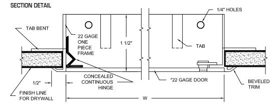
The WB DW-PF Press-Fit door is a unique lightweight door that installs easily by bending the tabs on the return back to grip the drywall. The frame, return and doorstop are one-piece construction with a beveled frame resulting in an attractive finished look.
