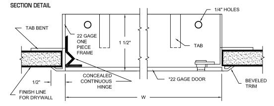
The WB PF Press-Fit door is a unique lightweight door that installs easily by bending the tabs on the return back to grip the drywall. The frame, return and doorstop are one-piece construction with a beveled frame resulting in an attractive finished look.
